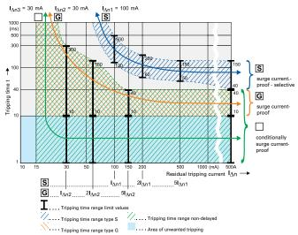
**IEC 60364-4-41** deals with additional protection: The use of RCDs with a rated residual operating current not exceeding 30 mA, is recognized in a.c. systems as additional protection in the event of failure of the provision for basic protection and/or the provision for fault protection or carelessness by users.
