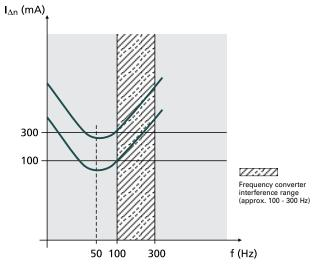
Frequency converters are used in a wide variety of systems and equipment requiring variable speed, such as lifts, escalators, conveyor belts, and large washing machines. Using them for such purposes in circuits with conventional residual current devices causes frequent problems with unwanted tripping.
